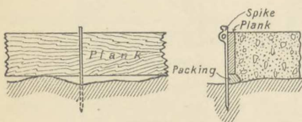
FIG. 133.—Moulds for Concrete Foundation.
