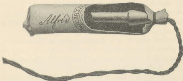
FIG. 79.—Electric Detonator Fuse inserted in Cartridge.
