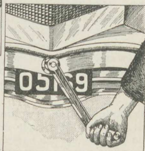
Wrong method of holding starting handle (right).
