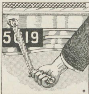
Correct method of holding starting handle (left).
