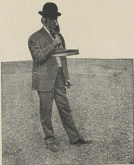
FIG. 141.—Wireless telephone receiving apparatus (induction method).
