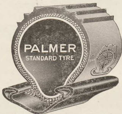
Fig. 30. —Palmer Beaded-edge Tyre
